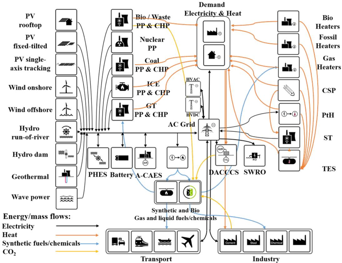
Figure A2: Schematic of the LUT Energy System Transition Model comprised of energy converters for electricity and heat, storage technologies, transmission options, and demand sectors<sup>3</sup>.
