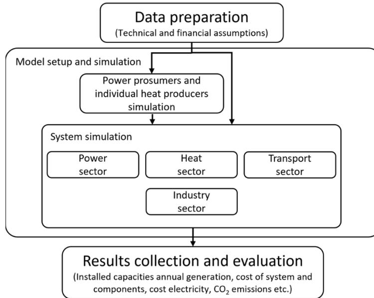
Figure A1: Fundamental structure of the LUT Energy System Transition model<sup>3</sup>.
